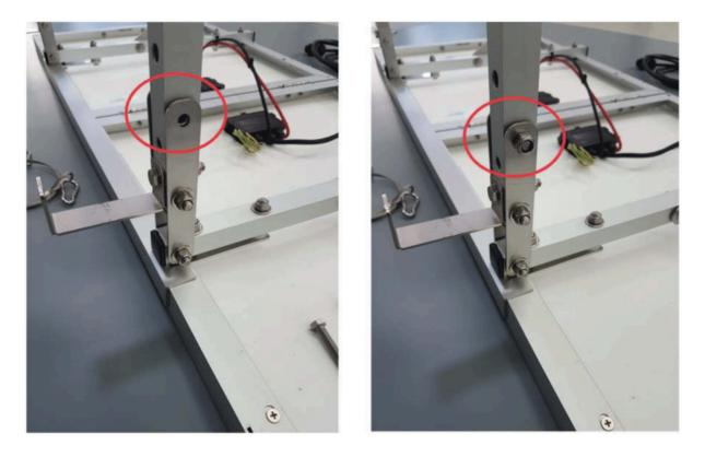
Put the bold and nut back in the marked hole and screw tight. Do this for both brackets.
